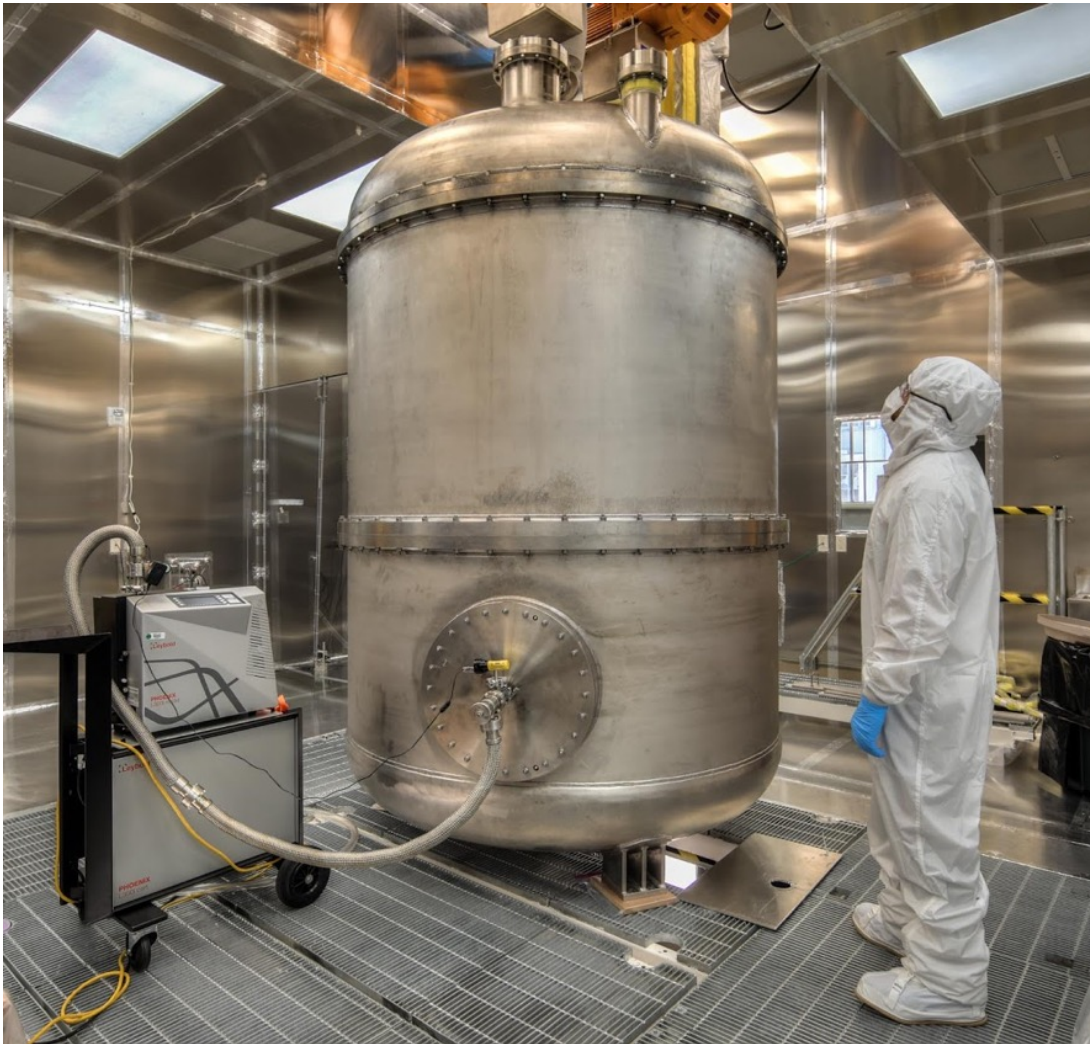
LZ Cryostat undergoing leak checks in SURF Surface Laboratory
